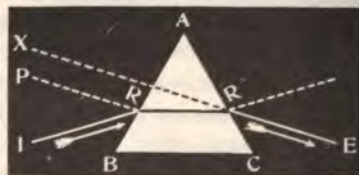
FIG. 145.—Refraction by a Prism.
